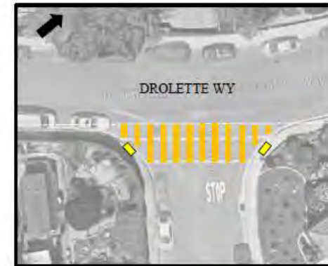
DROLETTE WAY AND CHERYL DRIVE SCOPE: HI VIS CROSSWALKS AND ADA CURB RAMPS
