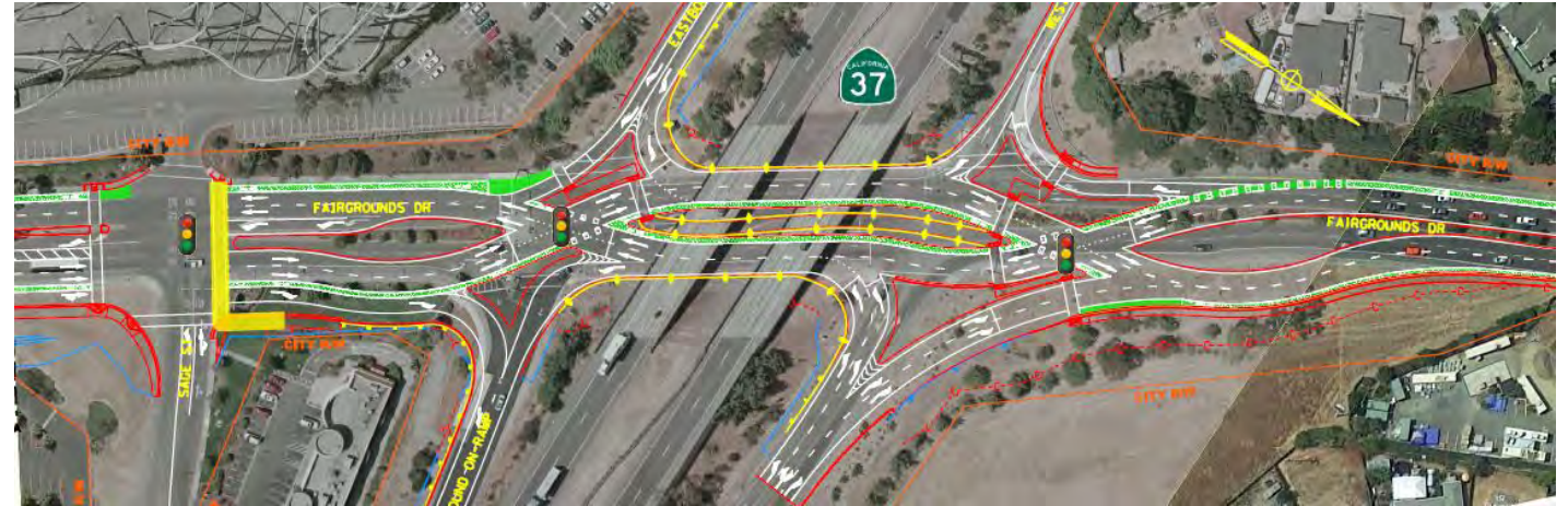
Fairgrounds Dr Divergent Diamond Interchange
