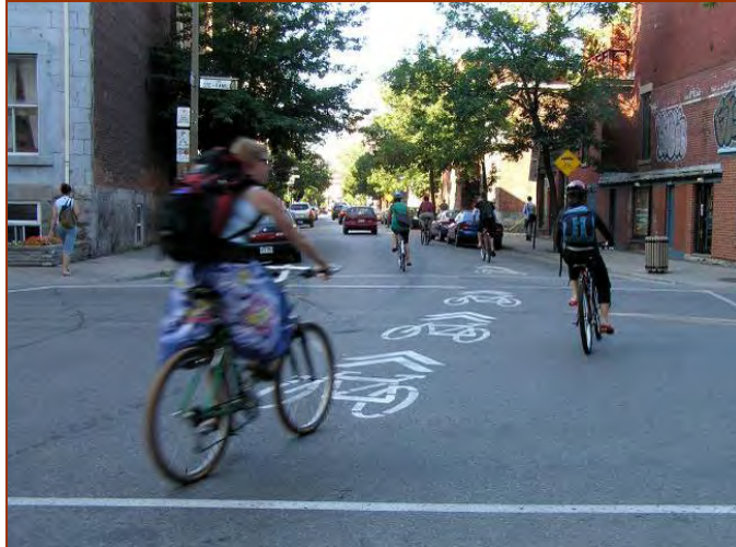
Photo: Bicycle lane markings across an intersection
