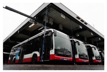
Figure 9. Example of Depot boxes Suspended from a Gantry Structure
