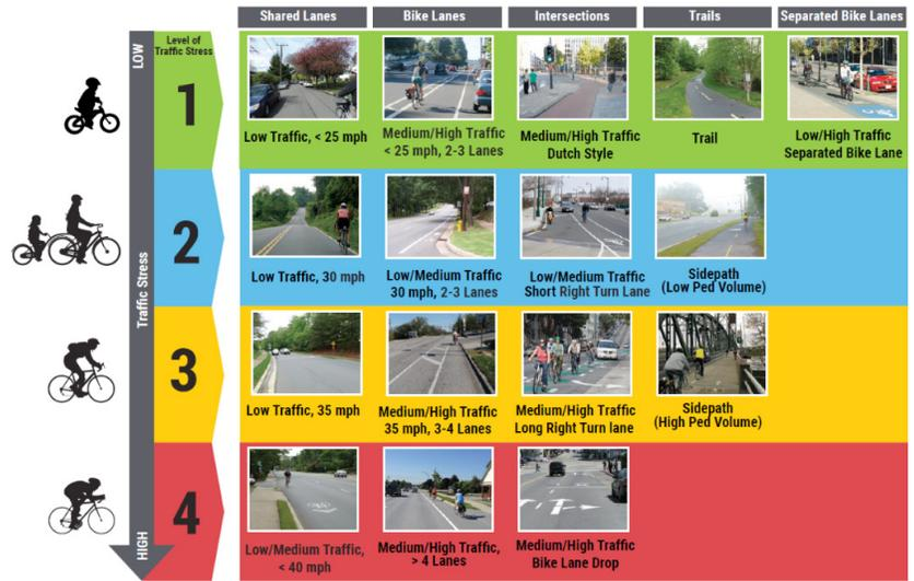
Figure 2. Level of traffic stress by bicycle facility
