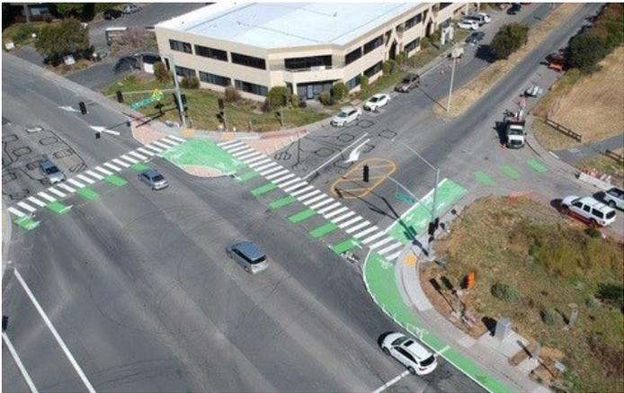
Figure 1. Rapid installation bicycle and pedestrian crossings at the intersection of Central Avenue and Rydin Road in Richmond, CA
